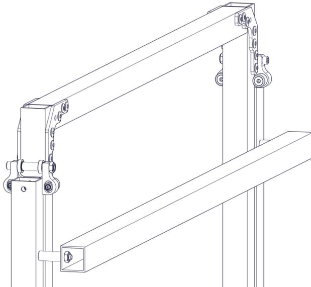
Do NOT make this assembly too tight! The inner carriages should freely and smoothly move inside the outer frame. If this proves too challenging to assemble in this fashion, you can remove the cam followers on one side to remove the inner carriage and then replace it when completed.
