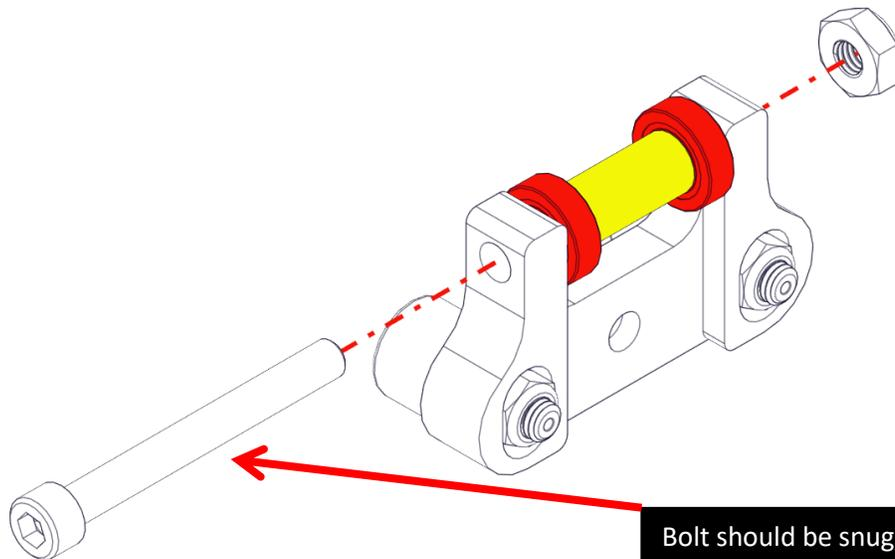
Bolt should be snug, but do not overtighten! The bearings need to freely roll.
